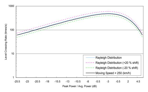
Figure D.2-8 Level crossing rate (Moving Speed = 250 km/h)
