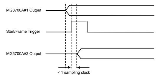
Figure C.1-5 Synchronization relationship of baseband signals when using Master/Slave
