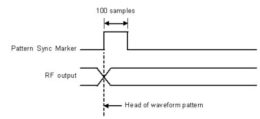
Figure 3.5-1 Pattern Sync Marker signal and RF output
