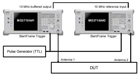
Figure C.2-1 Multiple MG3710A connection (external Start/Frame Trigger)
