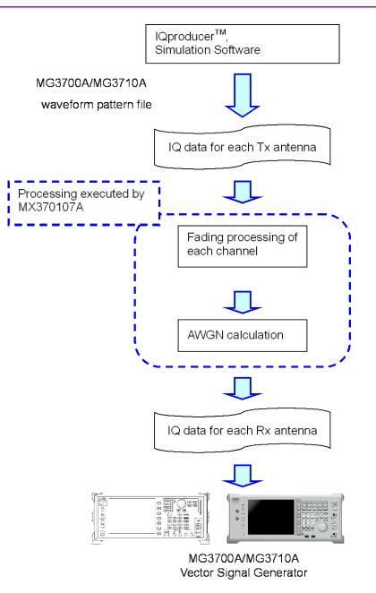
Fig. 1.1-1 Fading processing flow
