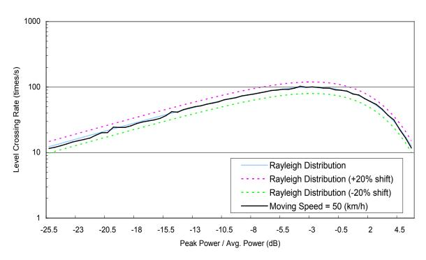
Figure D.2-4 Level crossing rate (Moving Speed = 50 km/h)
