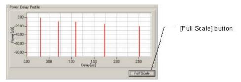
Figure 3.1.3-6 Power Delay Profile graph
