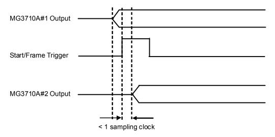
Figure C.2-5 Synchronization relationship of baseband signals when using Master/Slave
