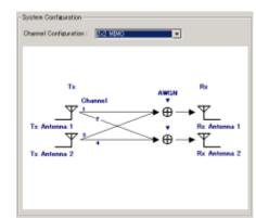
Figure 3.3.5-1 System Configuration (2 × 2 MIMO)
